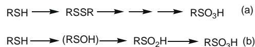
Scheme 1. Suggested reaction pathways for the formation of sulfonic acids by thiol oxidation.
